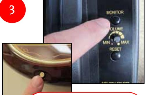
Make sure the clock functions properly by pressing the MONITOR button, which is usually located on the side, the front, or the bottom of the clock, to make sure the clock plays the melodies and performs the Magic Motion.
