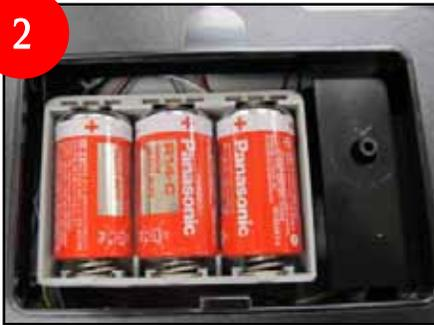
Make sure to insert all batteries properly into the battery holder, usually located on the back or bottom of the clock.
