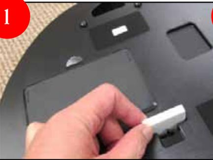
Some clocks come with a foam piece in the back to stabilize the pendulum during shipping. Please remove it to free the pendulum.
